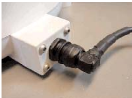
Figure 22 – Antenna Cable Connector Protection
